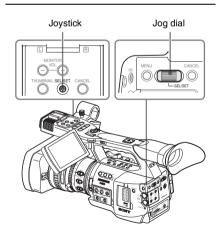
1 Tilt the joystick or turn the jog dial to set the cursor to "Date/Time" then press the joystick or dial.
